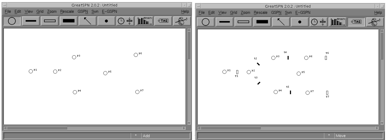
Figure 2.4: Place layout of the Readers–Writers model of Fig. 2.1 Figure 2.5: Place and transition layout of the Readers–Writers model
