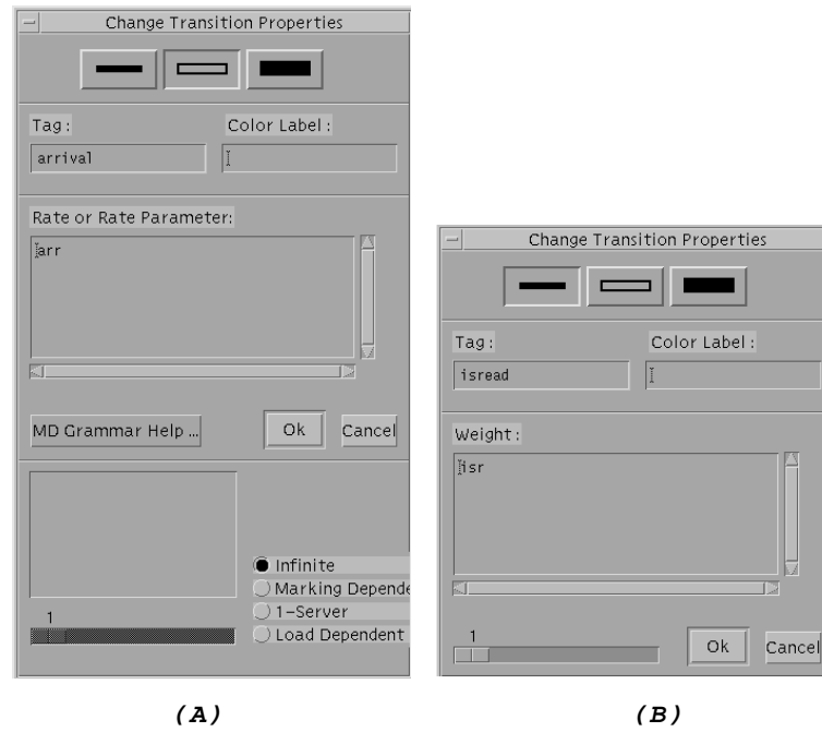
Figure 2.15: Windows for defining/changing properties of timed (A) and immediate (B) transitions.
