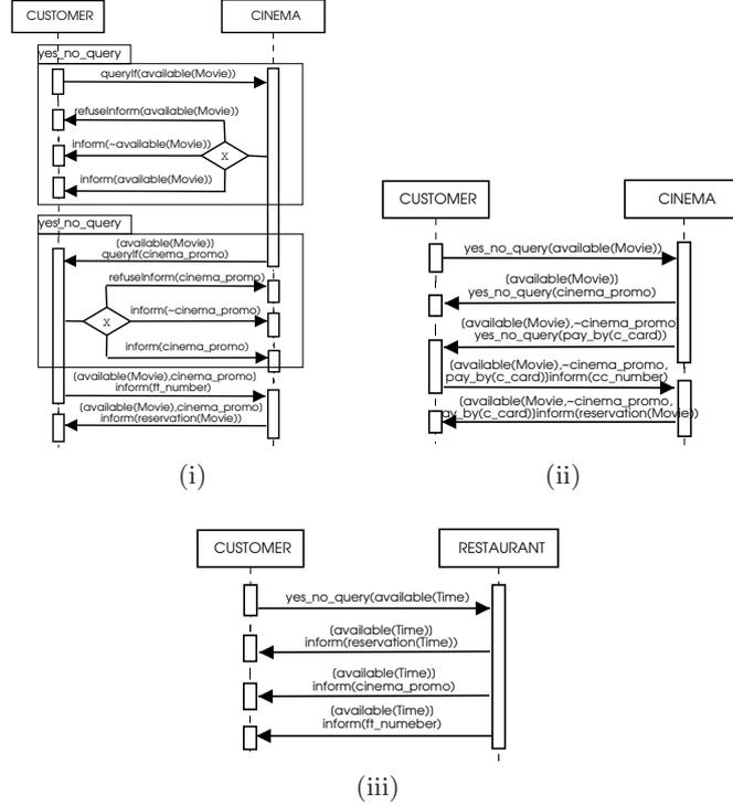
**Fig. 2.** AUML sequence diagrams representing the interactions between customer and provider: (i) and (ii) are followed by the cinema service, (iii) is followed by the restaurant. Formulas in square brackets represent preconditions to speech act execution
