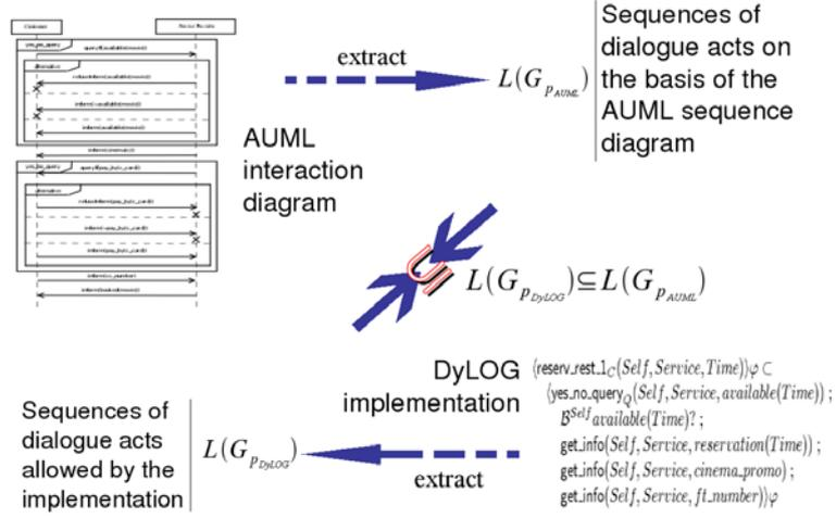
**Fig. 3.** Conformance verification of a DyLOG implementation w.r.t. an AUMI protocol: the problem is interpreted as the verification of language inclusion
