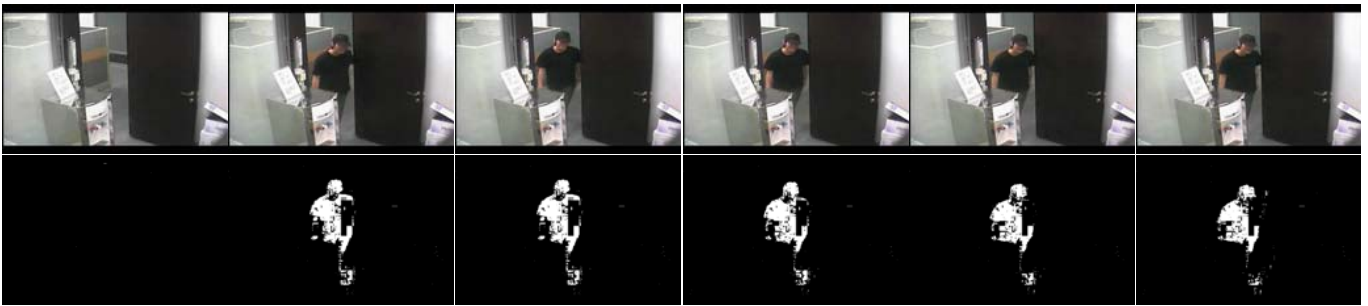
Fig. 4: Experiment 3. The left most column shows a background frame on the top and its result after change detection at the bottom. The top row from second to the right shows a sequence of input frames of a CCTV photage. The bottom row shows its corresponding resultant frames with change detected in white.
