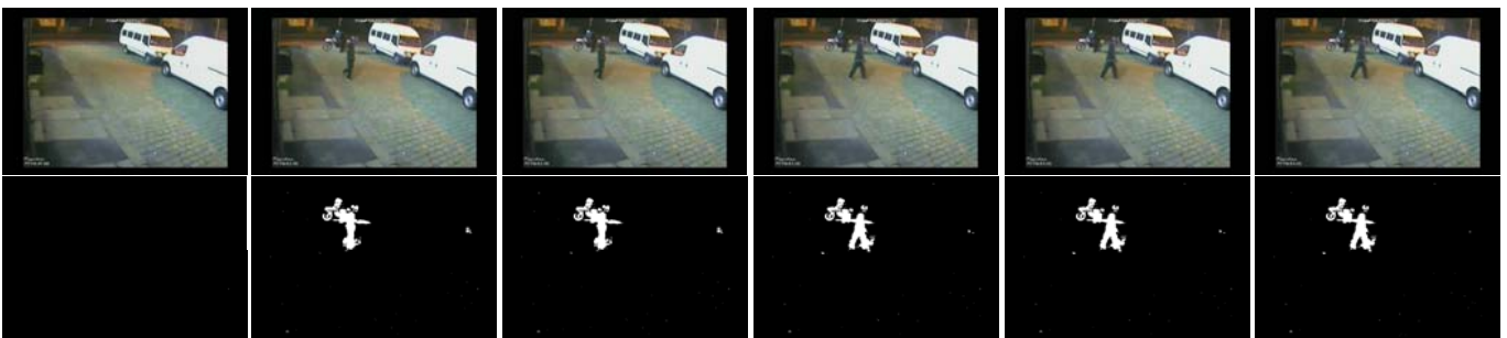
Fig. 5: Experiment 4. The left most column shows a background frame on the top and its result after change detection at the bottom. The top row from second to the right shows a sequence of input frames of a CCTV photage. The bottom row shows its corresponding resultant frames with change detected in white.
