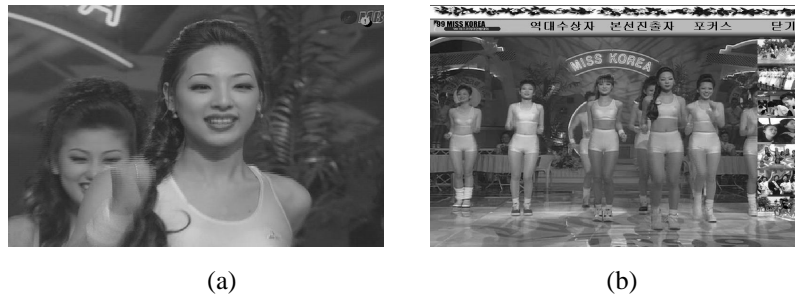
Figure 3. An example of MPEG-4 applications for interactivity. (a) shows the main program, Miss Korea 99, with MPEG-2 A/V and (b) shows the output of interactivity with MPEG-4 technology at a user's request (additional photos are displayed by clicking additionally focused photos, one of the menu on the top of the screen).
